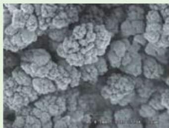
ProSwift WAX-1S Monolith (Magnification 5000x)
